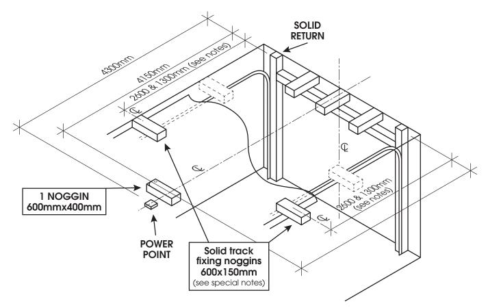
**NOTES:** Doors higher than 2405mm high up to 3190mm high and all wind rated, insulated or special P7D doors will require two intermediate fixings at 1300mm.
